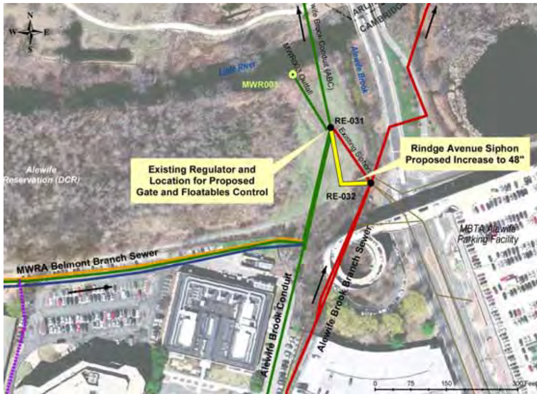
Figure 6: Control Gate and Floatables Control at Outfall MWR003 and MWRA Rindge Ave. Siphon Relief
