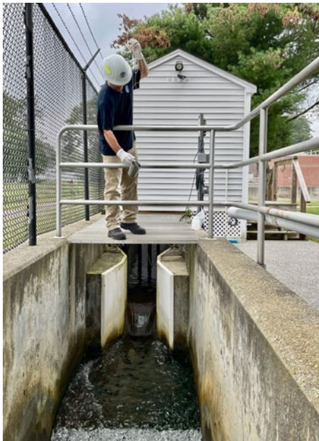
Figure 3: Collecting PFAS samples at the Clinton Wastewater Treatment Plant
