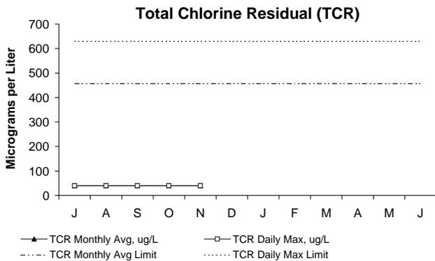
In November, both the maximum daily and monthly concentrations of TCR were below permit limits. TCR, or Total Chlorine Residual in the effluent, is a measure of the amount of chlorine that remains after the disinfection/dechlorination process. If the chlorine residual in the effluent is too high, it may threaten marine organisms.
