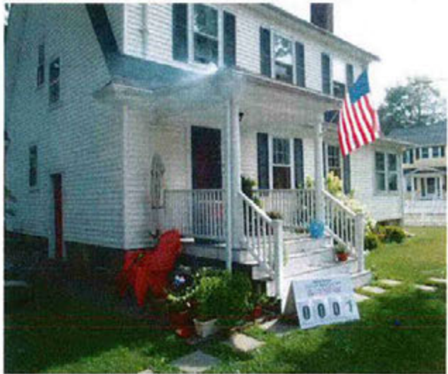
Smoke Testing Confirms House Downspout is an Inflow Source Connected to the Sewer
