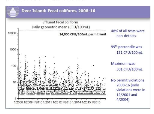
Samples are taken 3x/day. Samples are taken at the tail end of the disinfection basin, so after chlorine has been added and before it goes into the outfall.
