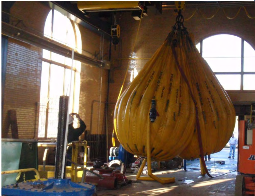
Load Testing of Hoist
