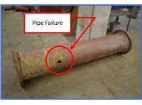
Existing Primary Sludge (PSL) and Primary Scum (PSC) lines are leaking due to failed glass lining and pipe corrosion
