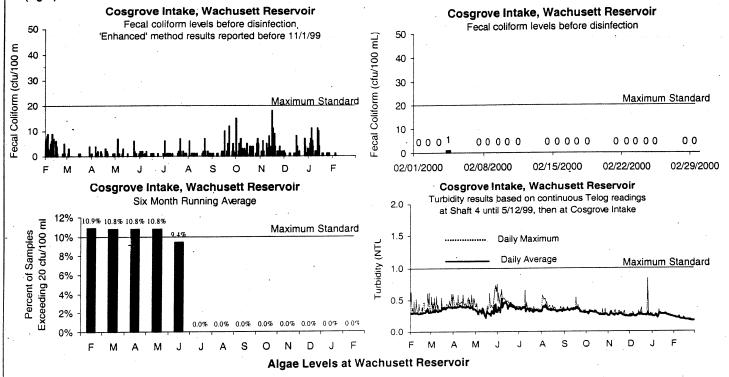
Taste and odor complaints at the tap are usually due to algae, which originate in source reservoirs, typically in trace amounts. Occasionally, a particular species grows rapidly, increasing its concentration in water. When *Synura, Anabaena*, or other nuisance algae blooms, MWRA treats the reservoirs with copper sulfate, an algaecide.
