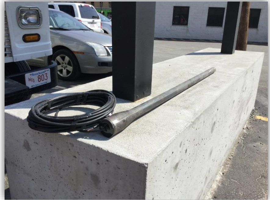
5 Foot Anode Prior to Installation
