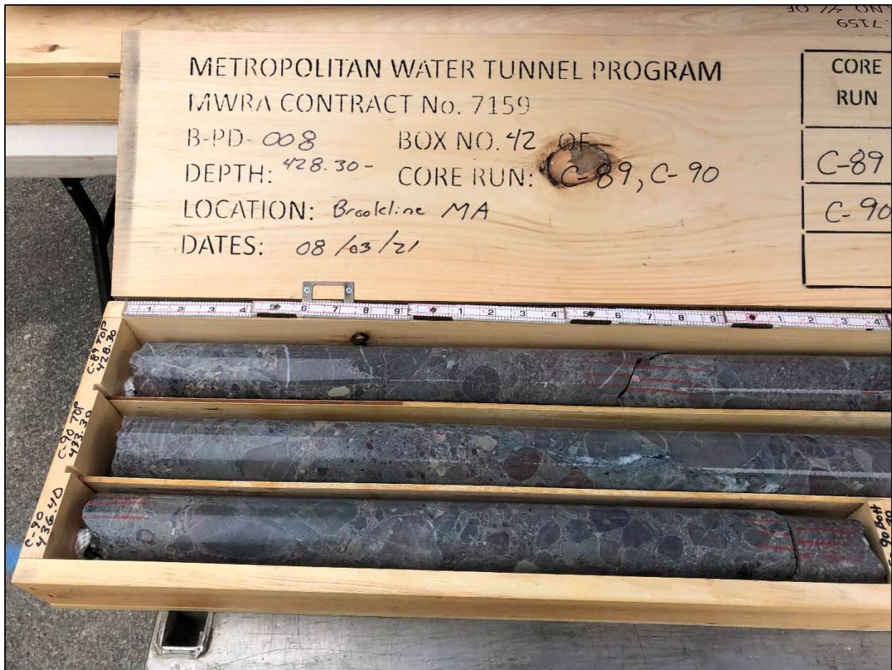
Figure 2. Typical Rock Cores Extracted from a Boring.
