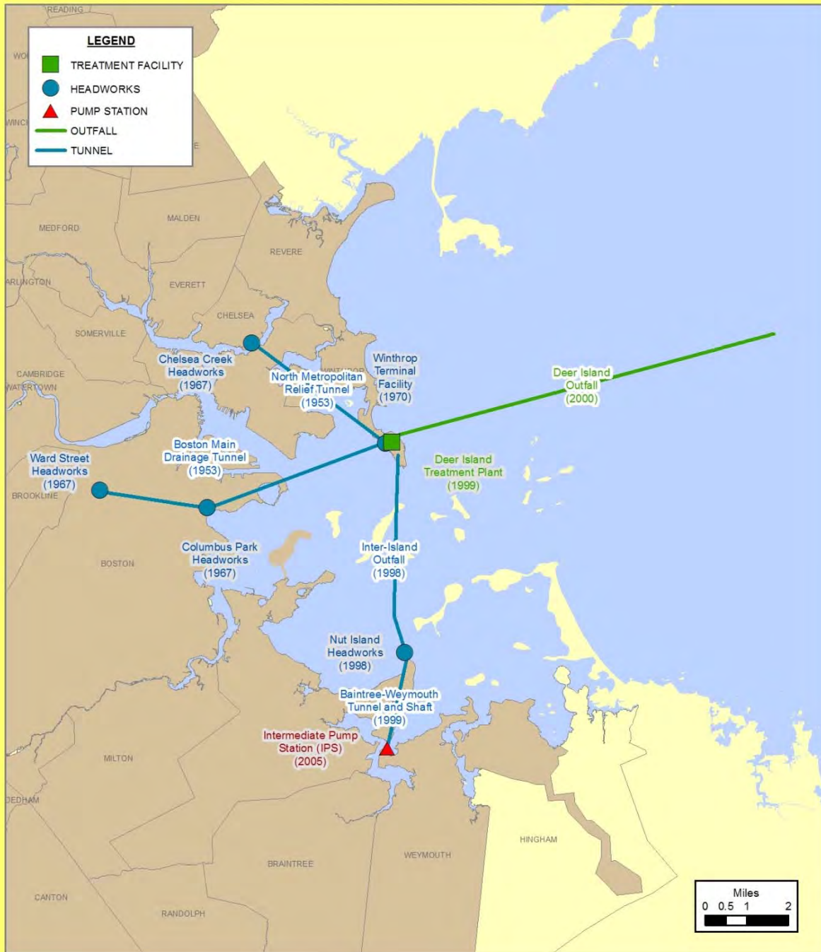
FIGURE 8-1 Headworks & Harbor Tunnel Location Plan
