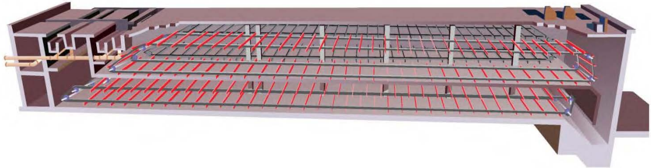
Figure 6-5: Stacked Primary Clarifier 1
