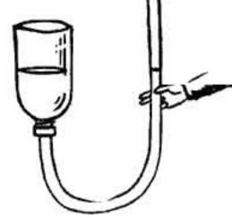
4. Slowly lower the end of the tube. When the water level just reaches the end of the tube, put your finger firmly over the end.
